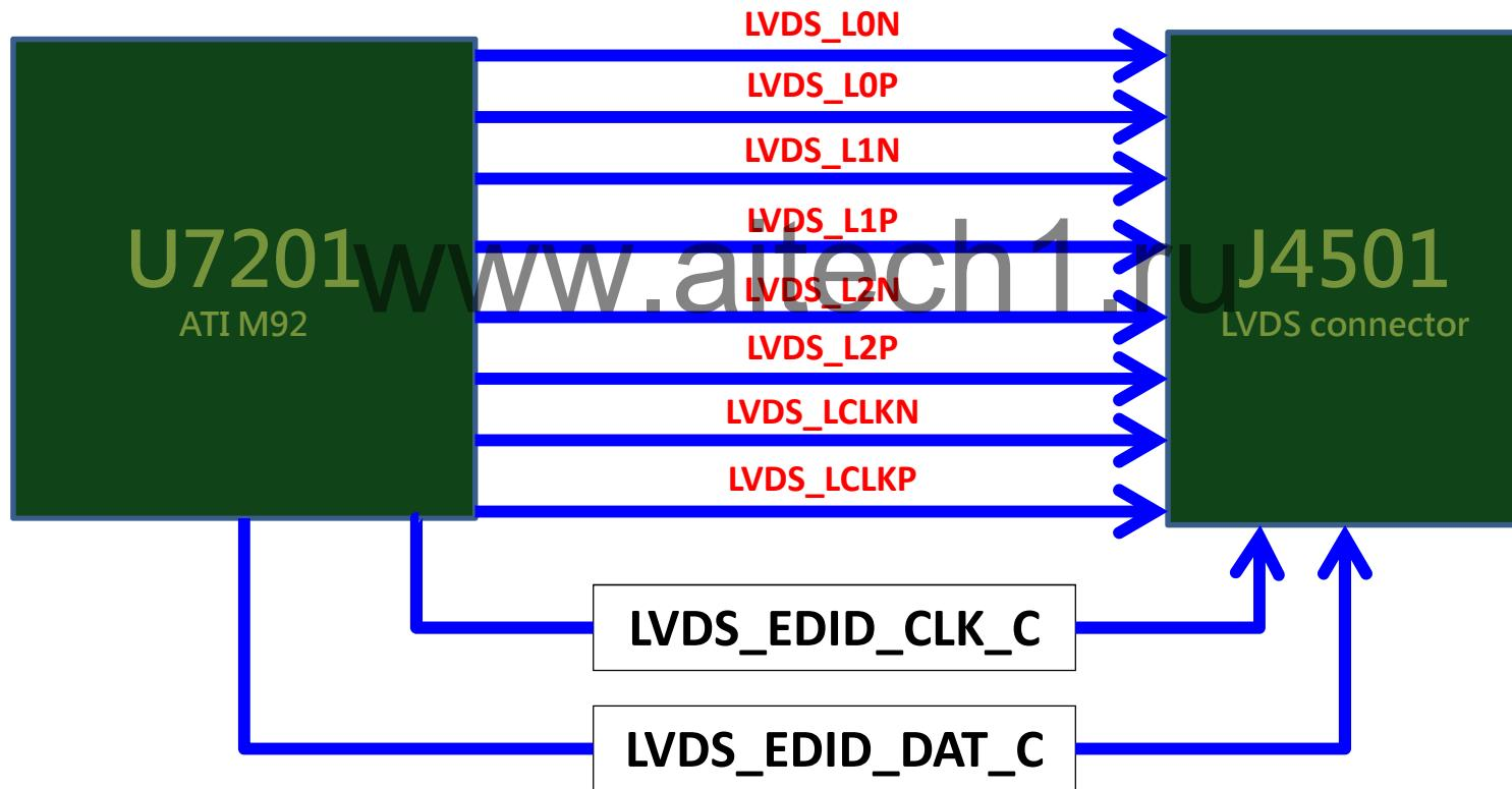
➤ Connection problems between GPU and display devices
