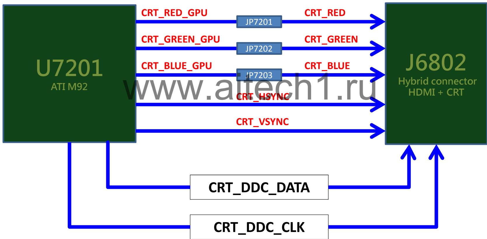
➤ Connection problems between GPU and display devices
